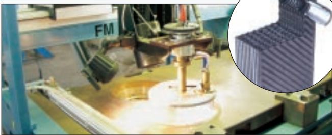
Plate T (hard) – lower heat transfer and lower pressure loss
